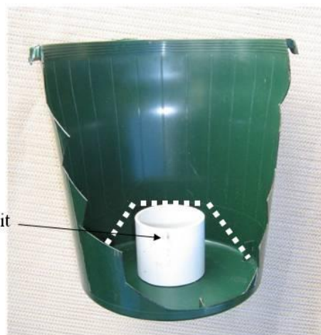
Entire conduit section glued in place over the central collar. Dotted line indicates the position of the capillary tape that, when in place (resting on an impervious plastic cover) will transmit drainage water from this pot to an upper one sitting in it (refer to the TWMS configuration).
