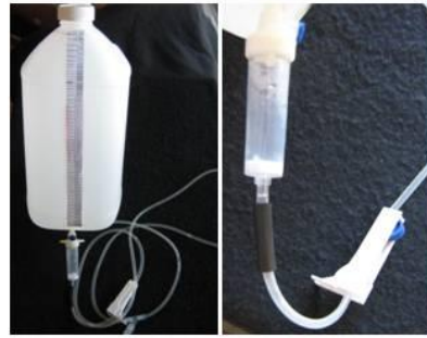
Infusion set, with filter and flow controller, connects valve to external reservoir.
