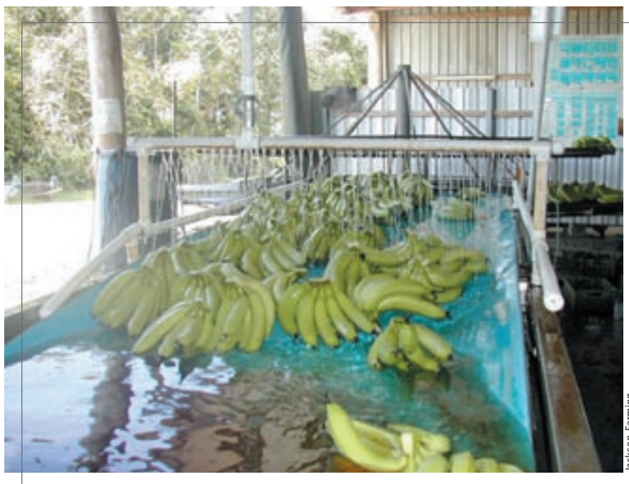
Jackson Farming's WaterWise project included the development of a system that recycles and treats 100% of the water used in bunch and fruit washing – saving a massive seven million litres of water a year.
